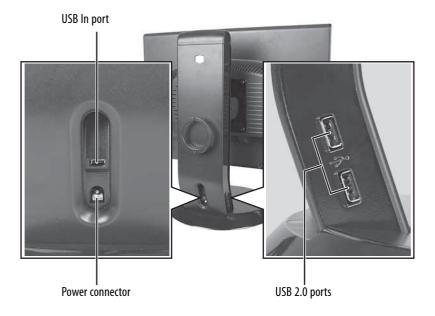
2 To provide full power to your stand's USB ports, connect the AC power adapter to the power connector on the back of your USB stand and into an AC power outlet.
